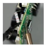
Once melted, wiggle and pull the component out from the other side with pliers or forceps. You can do this same procedure when inserting the new component as well but just make sure its heat long enough to wet properly or touch it up after its in position.
