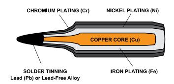
When you file the plating off, you dramatically reduce tip life by compromising its ability to melt solder and for solder to stick to it. Once you get through the plating, you'll have a hole in your tip and it will no longer work correctly.
