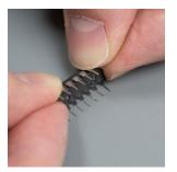
Now carefully roll the chip to straighten the pins between the body of the chip and hard surface. Do the same to the other side and then the chip should fit into the holes nicely.
