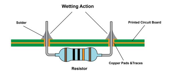
*The ideal solder joint should appear smooth and cone-shaped with a 40-70 degree wetting angle.*
