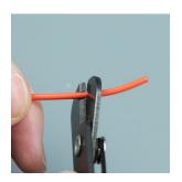
Using your wire strippers of choice, bite down on the insulation lightly to grip the insulation. Close down on the wire just enough to slightly pierce the insulation. This will come with experience for you to get a feel for it.
