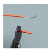
Score the wire by twisting the wire strippers around. With the jaws still locked on the insulation, squeeze a little bit and, pull up to remove the insulation cleanly.
