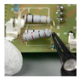
Somtimes component leads can get stuck by a little bit of solder that was left behind. If you can't seem to get the hole completely clean with any desoldering methods you can heat up the joint and try pulling the part out instead.
