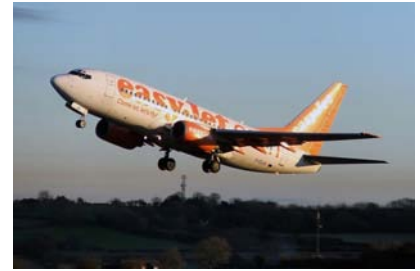
Figure C.11. Boeing 737-700: 30 kWh per 100 passenger-km. Photograph © Tom Collins.
