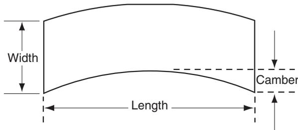
Figure 2 – Measurement of camber – Using straightedge
