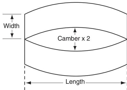
Figure 3 – Measurement of camber – Using two lengths
