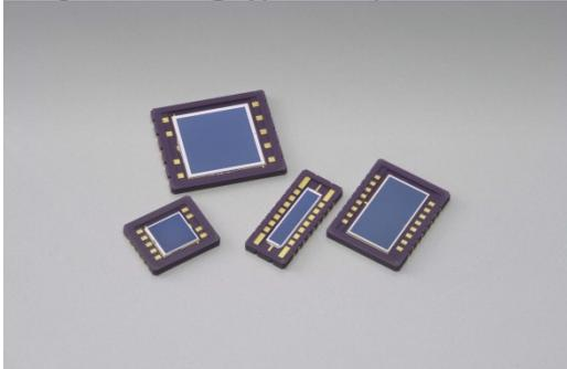
Do not touch the surface of silicone resin. Silicone resin is soft. Applying external force on it can cause scratches to its surface and short-circuit or breaks due to wire deformation.
