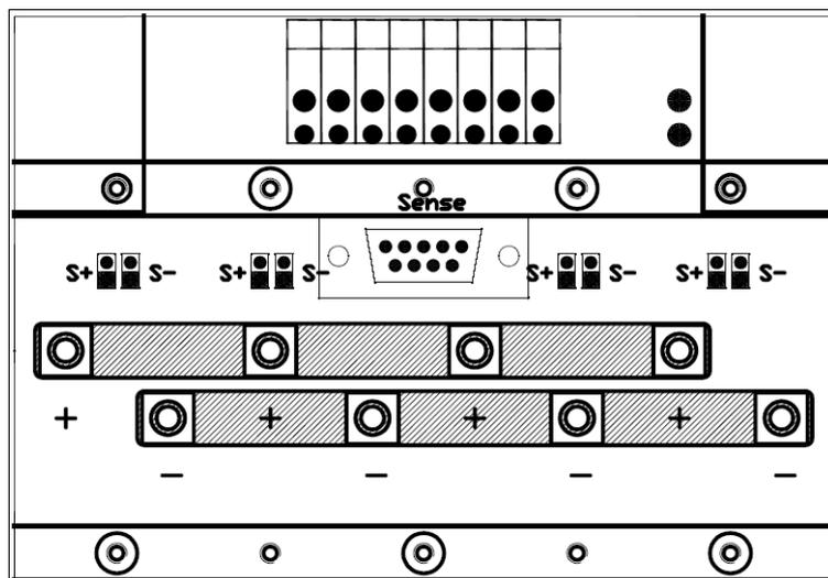
Figure 7.5: Four Channels Parallel
