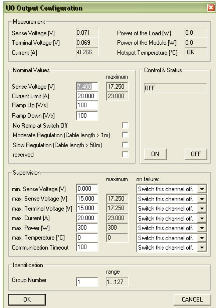
In this situations the advanced (PID) regulator of the *Moderate Regulation* should be used.
