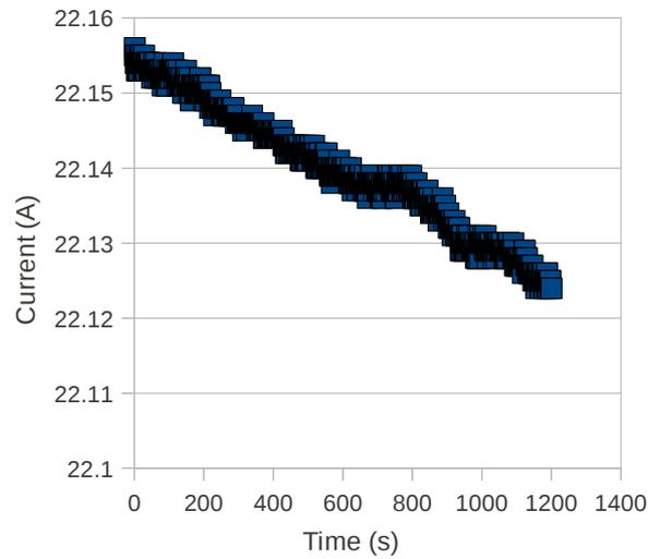
Fig 17: The excursion of current for channel 3 in the first 20 min (normal excursion)
