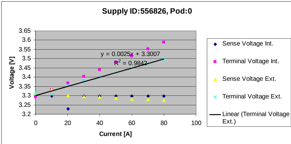
**Chart 2: Supply linearity under remote sense operations for 24V pods**
