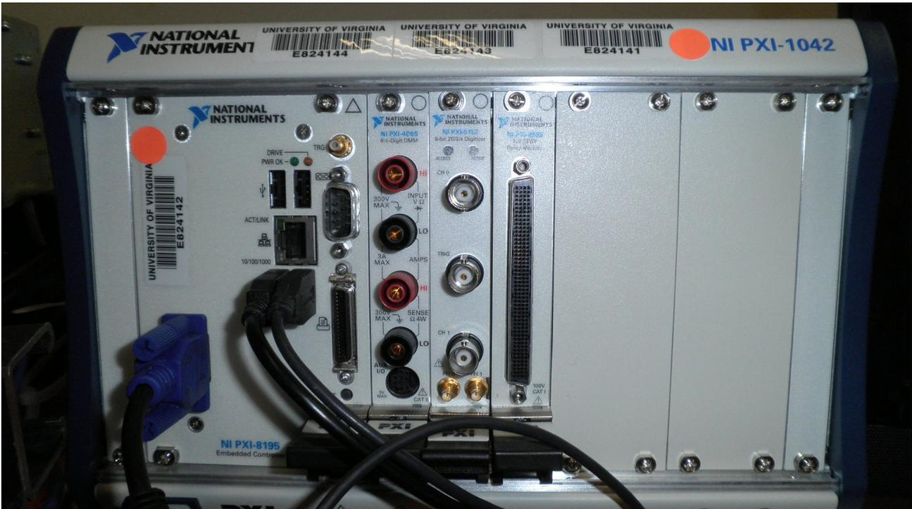
Fig 6: The front view of the PXI crate
