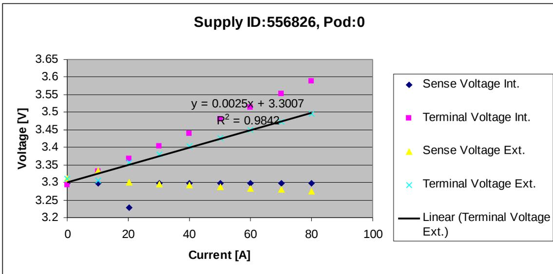
Chart 1: Supply linearity under remote sense operations for 3.3V pods
