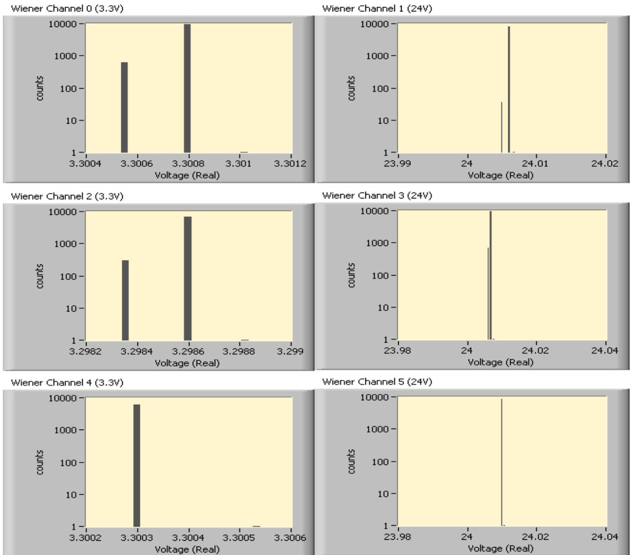
Fig 13: Histogram of the voltage stability test for all pods of 556829
