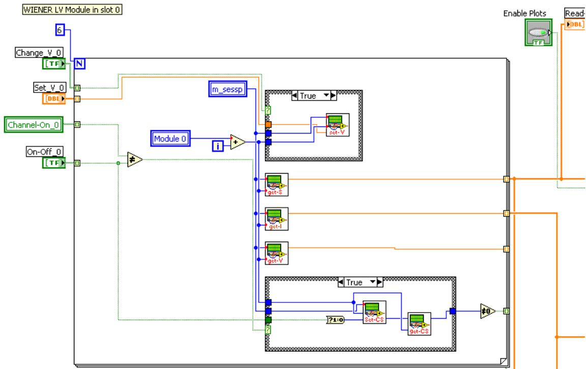
Fig 10: Block diagram for voltage stability test
