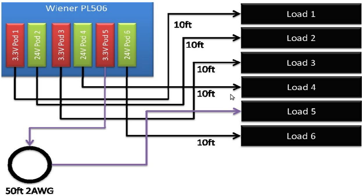
Fig 3: The topology of this configuration for the Wiener PL506 setup
