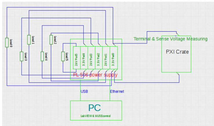
Fig 7: The sample diagram of the electrical set up
