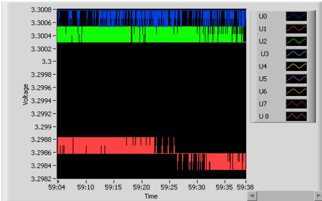
Figure 14: Strip chart of testing 3.3V channels for 556829
