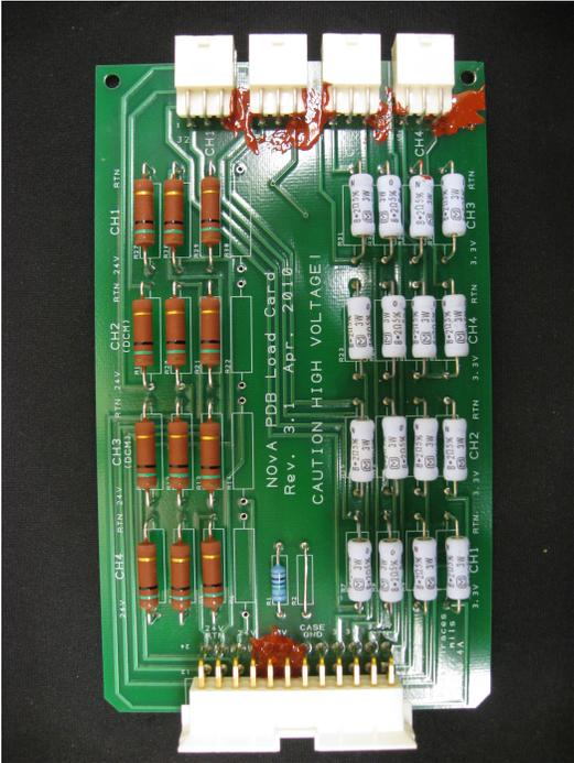
Figure 19. FEB load board used to put the backplane under load when testing the PDBs.
