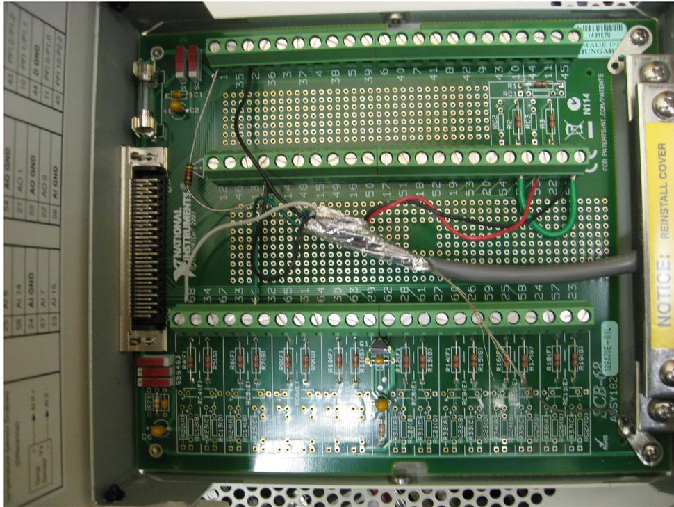
Figure 13. View of the SCB-68 terminal block with the cover removed.
