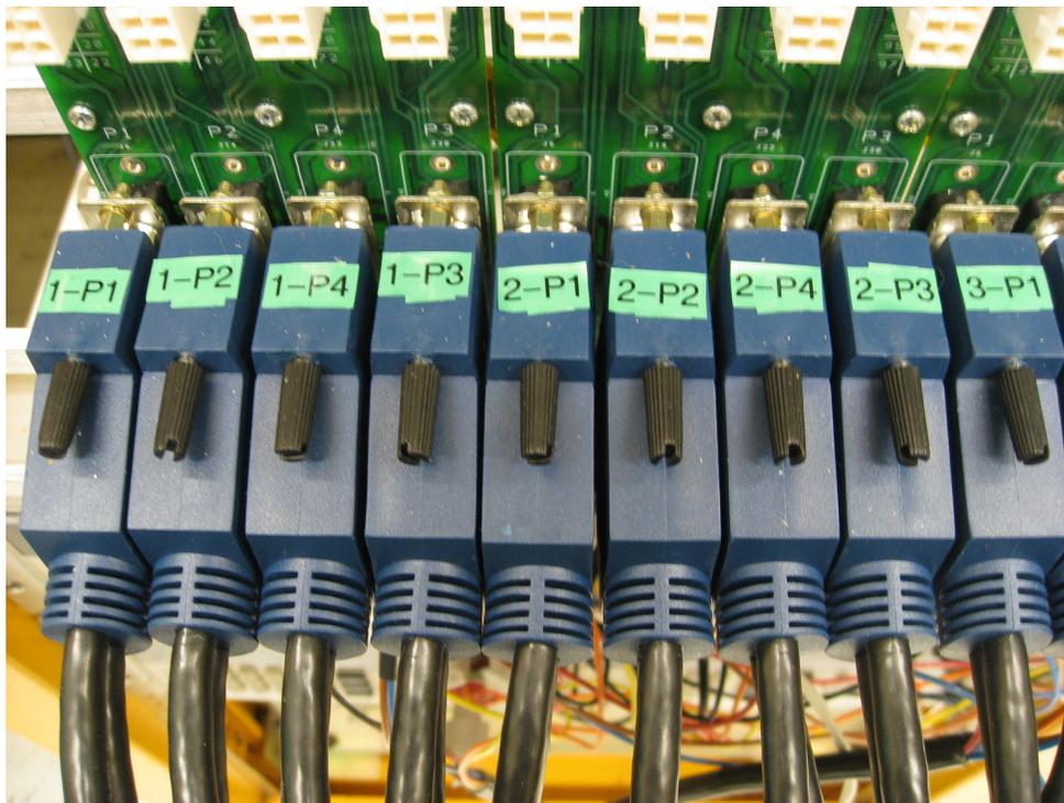
Figure 16. Numbering of the relay connectors on the Test Connector Boards. From left to right on each board it goes 1-2-4-3.
