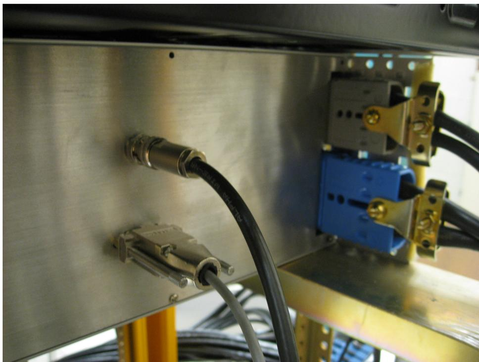
Figure 17. High voltage, sense, 3.3V, and 24V connectors on the back of a PDB.
