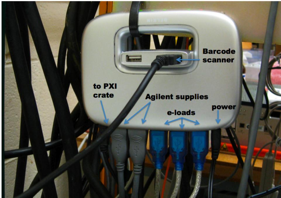
Figure 11. USB hub connecting the e-loads and the power supplies to the PXI crate.
