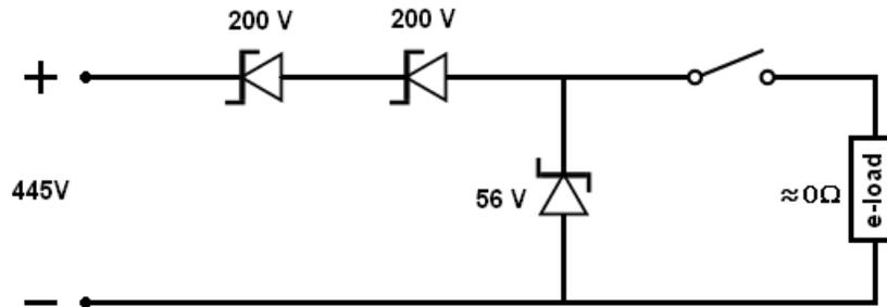
Figure 20. Current limiter test circuit.
