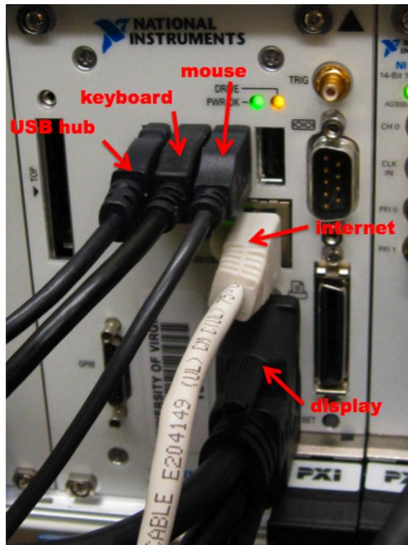
Figure 15. Closer view of panel on PXI crate showing USB connections.
