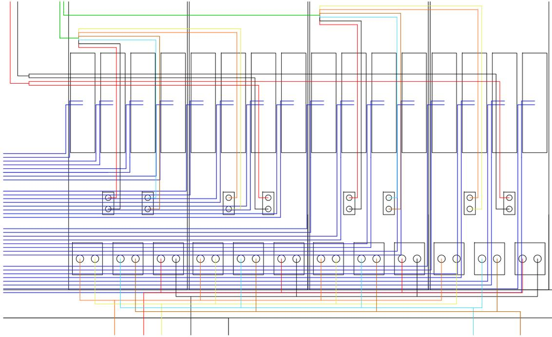
Figure 8. Close up of the PDB wiring showing the Test Connector Boards.
