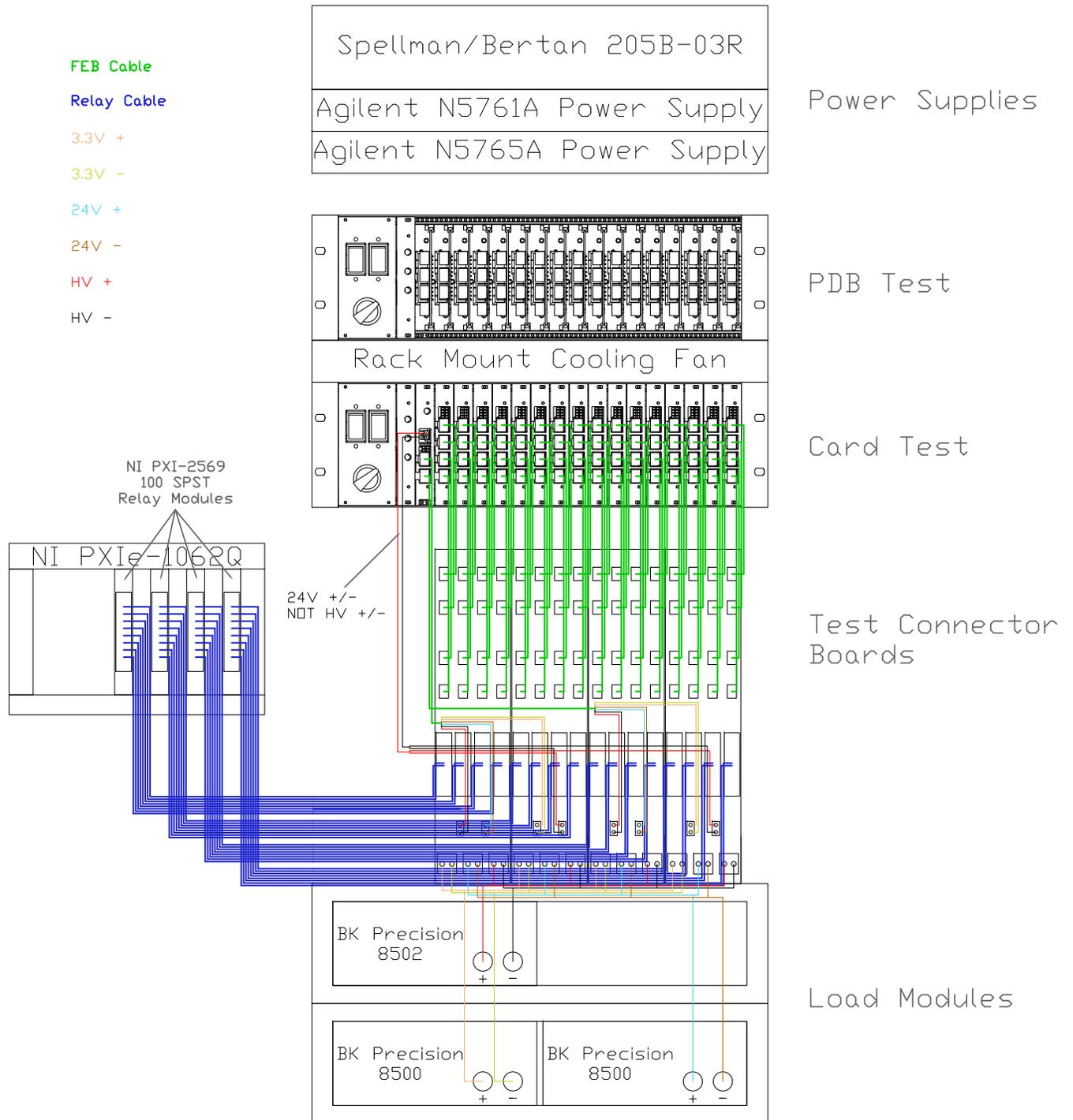
Figure 7. The PDB test rack showing the cable routing.
