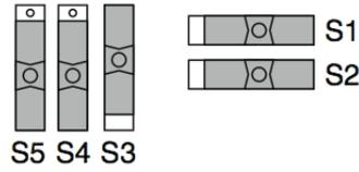
Figure 12. General purpose switch configuration for SCB-68 terminal block.
