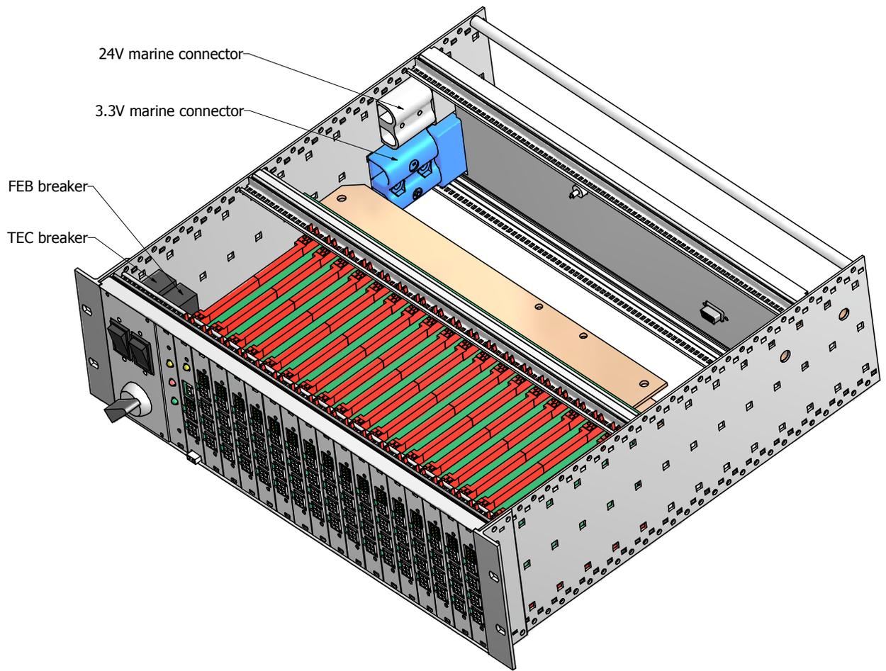
Figure 2. NOVA Power Distribution Box.
