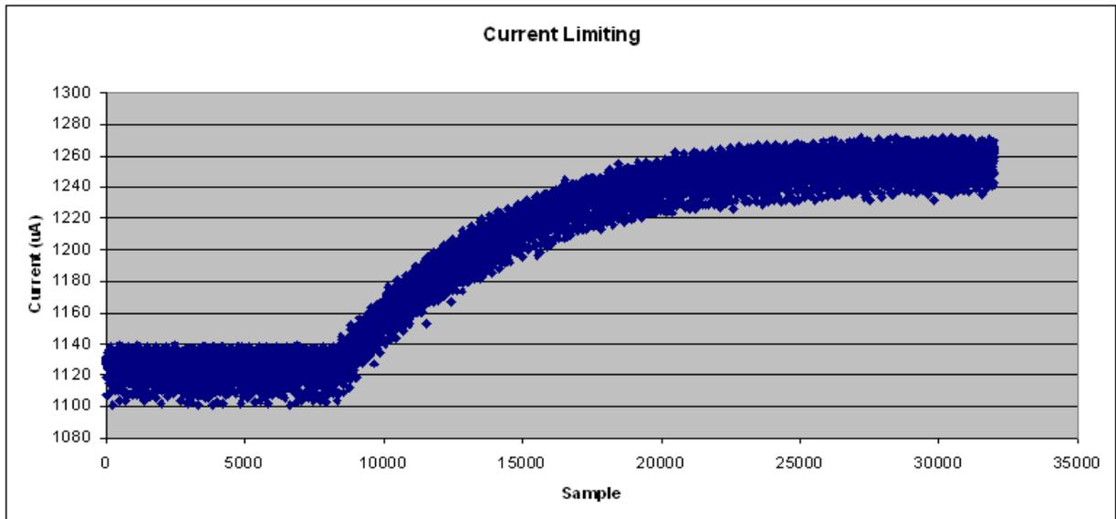
Figure 30. Graph of Current Limit data showing the response during a short. This is not automatically produced during testing.
