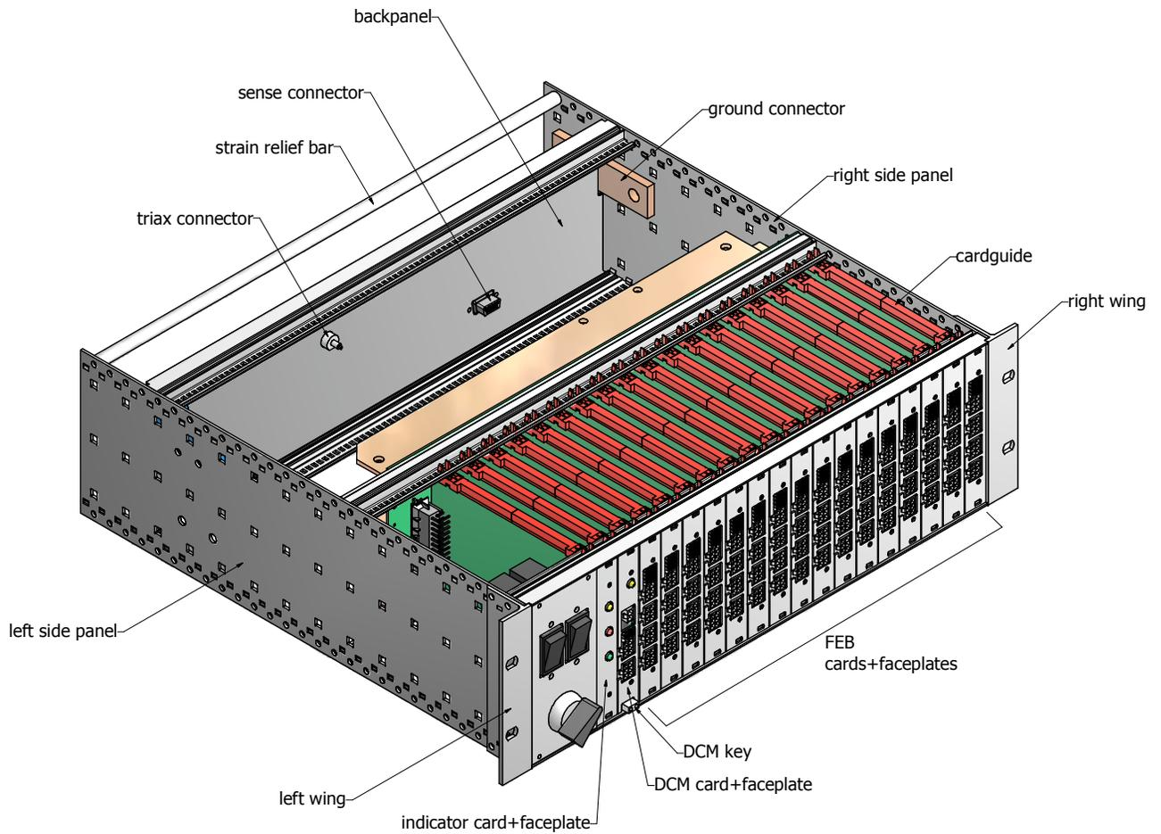
Figure 1. NOVA Power Distribution Box.
