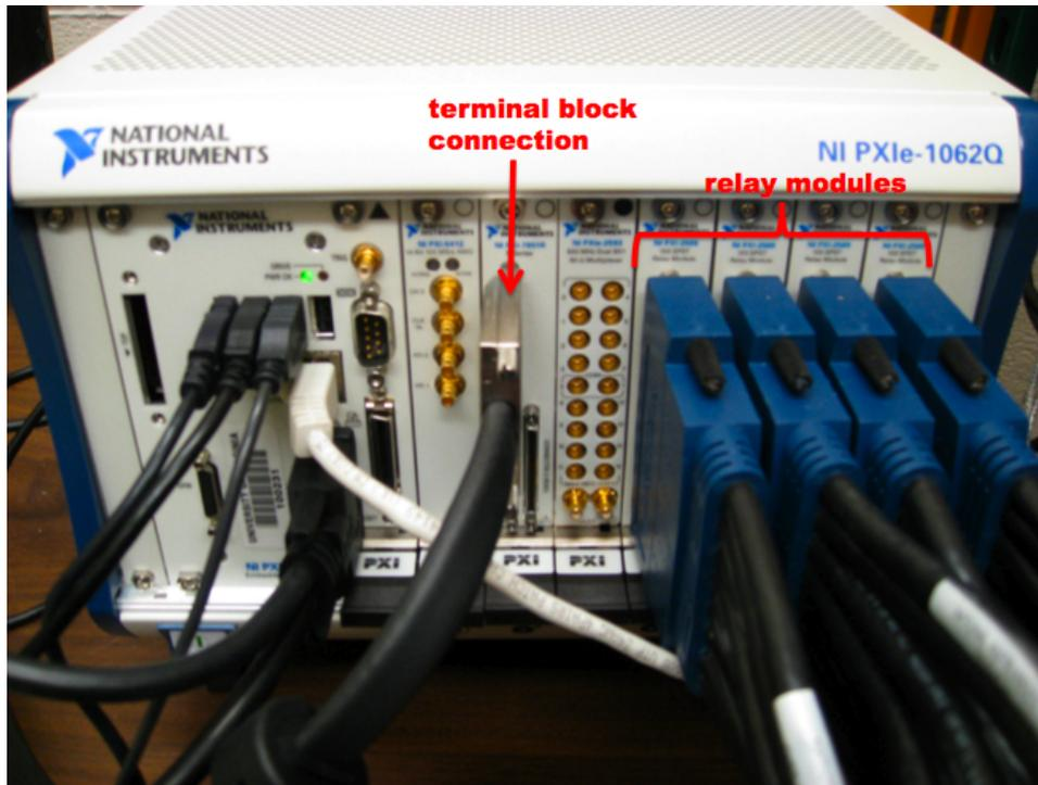
Figure 14. National Instruments PXI crate.
