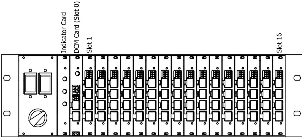
Figure 3. Numbering of the “slots”.
