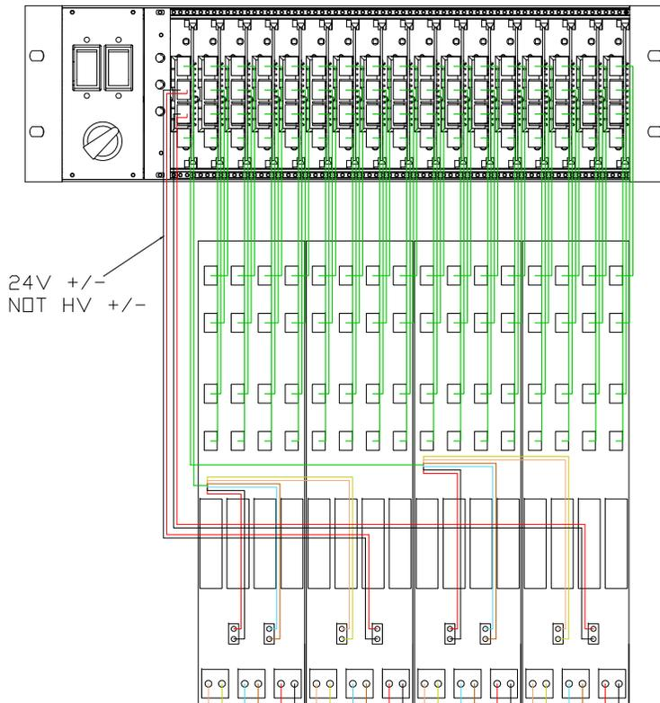
Figure 9. Cabling for load boards in upper PDB (prototype PDB and relays not shown).
