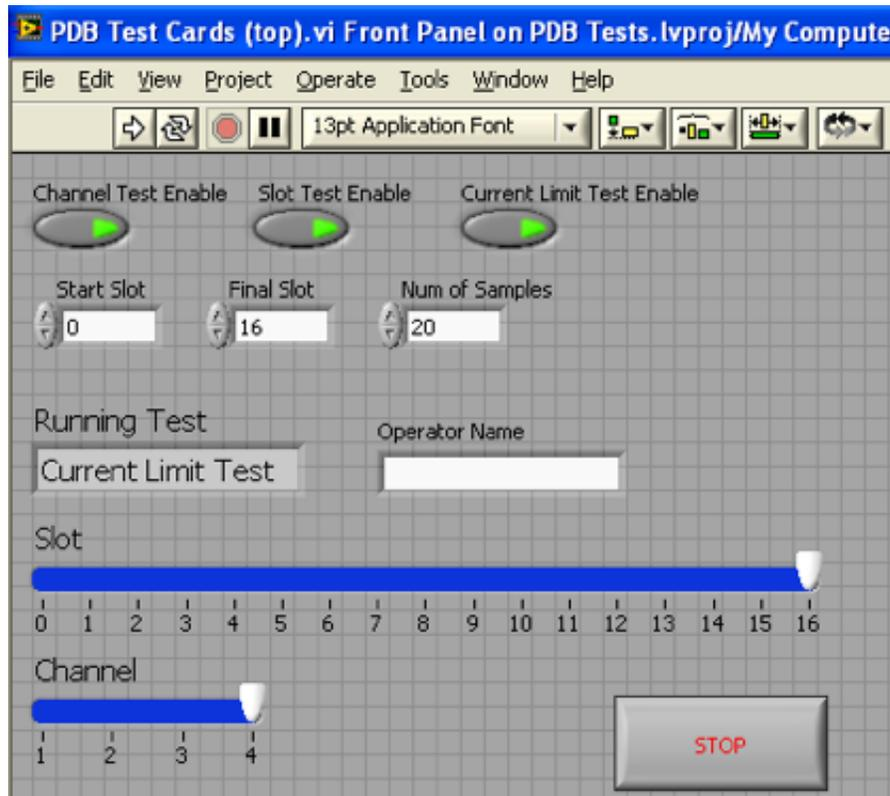
Figure 21. Test configuration and status graphical interface for the cards tests. The Start Slot, Final Slot, and Num of Samples controls apply to each of the three card tests. The green light on a test control indicates that it is enabled and will run once the run arrow is pressed.
