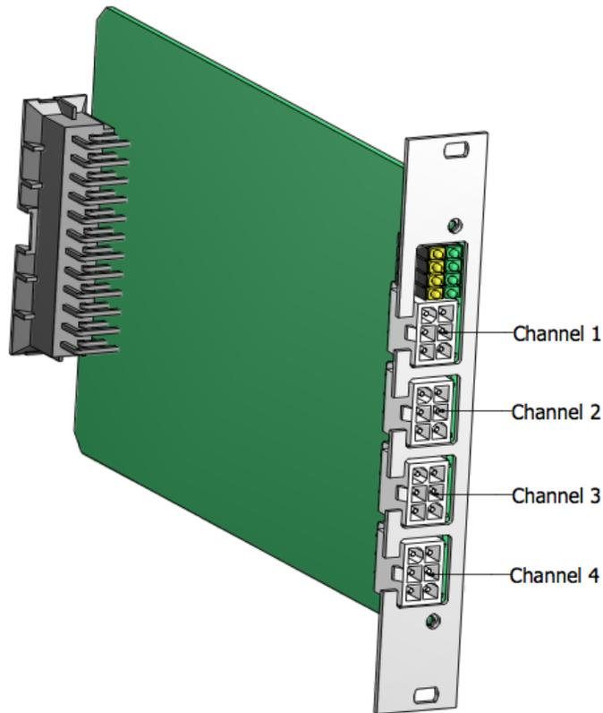
Figure 4. Numbering of the channels of an FEB card.
