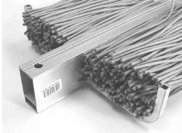
Picture shows 12" wide Cent-R-Rail cable tray with 3" load depth. The tray contains 520 4 UTP Category 5 cables (.21" OD).
