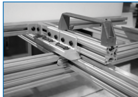
Panel measuring/in-feed table • Linear guide profile - 6.0" bearings
