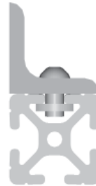
Slide pre-loaded part into T-slot
