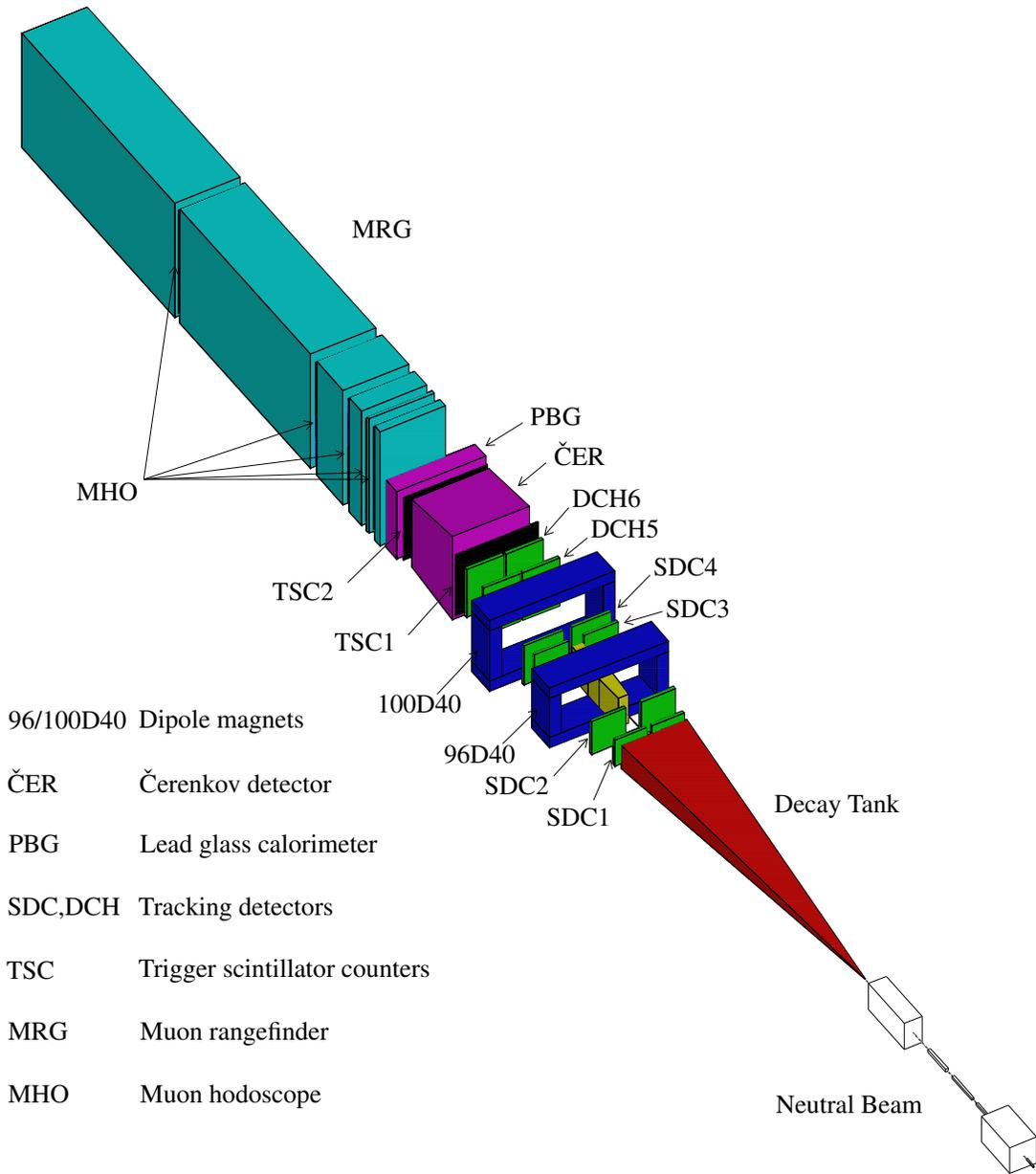
FIG. 17: E871 Experimental apparatus
