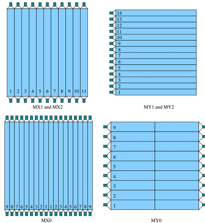
FIG. 30: Muon Hodoscope detector plane design
