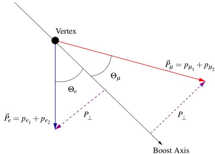
FIG. 46: Muon pair transverse momenta to electron pair transverse momenta sum relation through the collinearity angles  $\Theta_\mu$  and  $\Theta_e$
