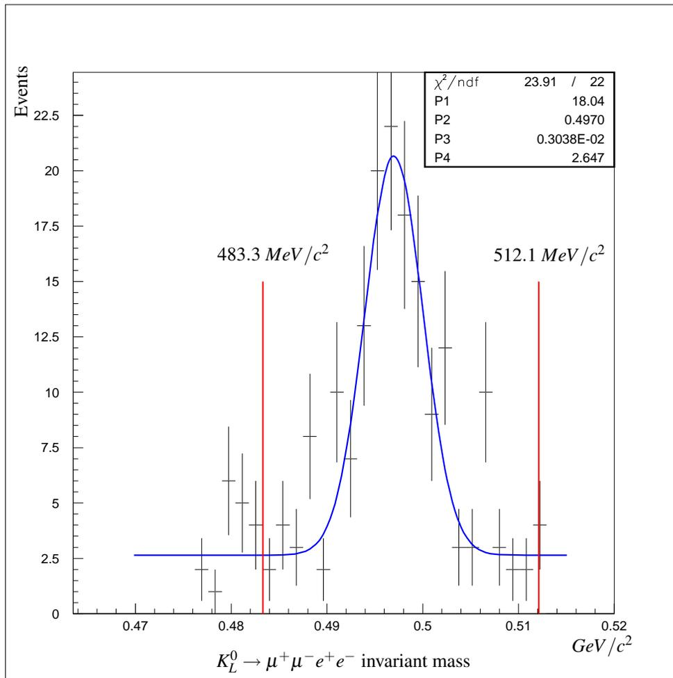
FIG. 50:  $K_L^0 \rightarrow \mu^+ \mu^- e^+ e^-$  invariant peak showing 171 events in the signal region composed of 119 signal and 52 background
