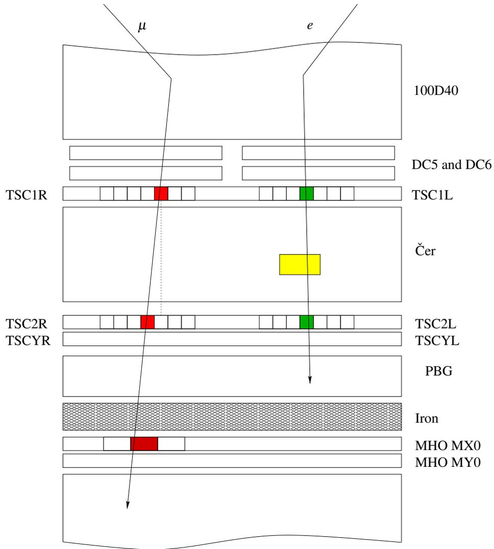
FIG. 32: Schematic overview of a level 1 event trigger
