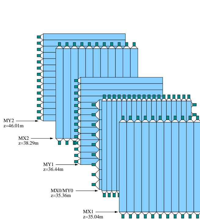
FIG. 29: Muon Hodoscope detector plane layout
