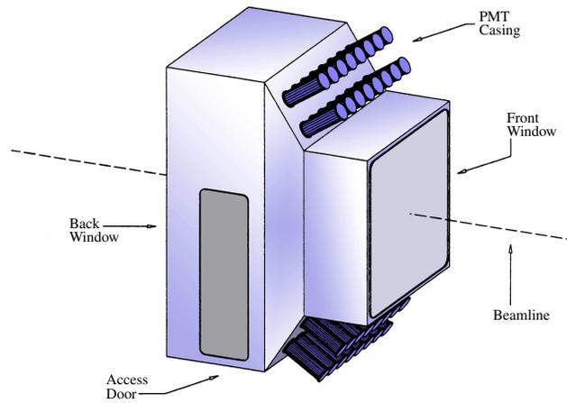
FIG. 24: E871 Čerenkov counter exterior geometry
