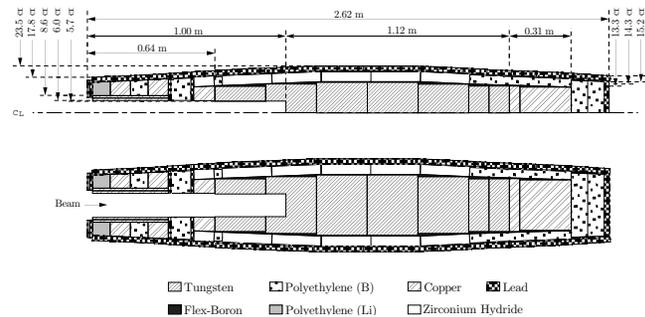
FIG. 21: Cross sectional view of E871 compact beam stop
