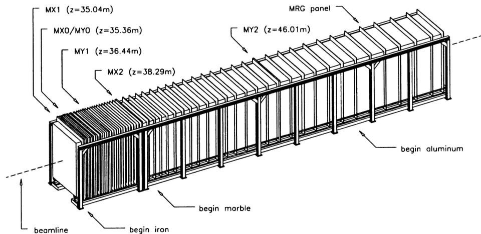
FIG. 28: E871 Muon ranger stack active detector placement
