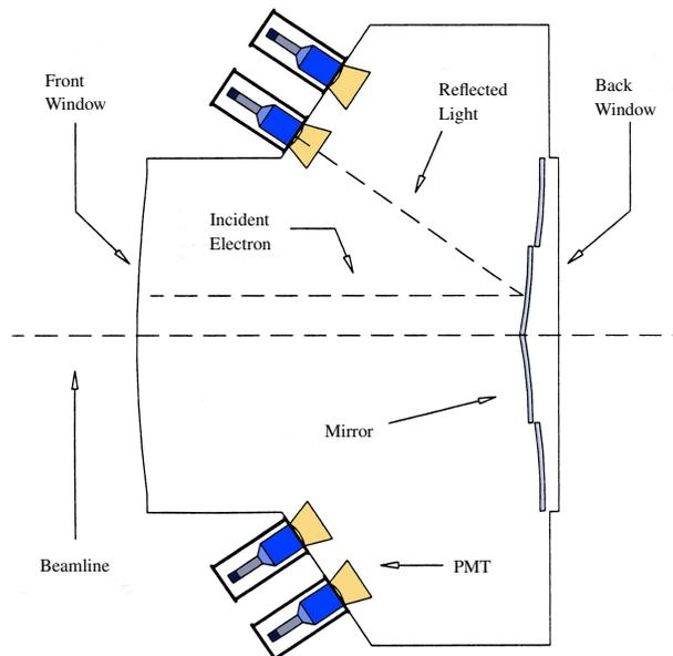
FIG. 25: E871 Čerenkov counter interior geometry
