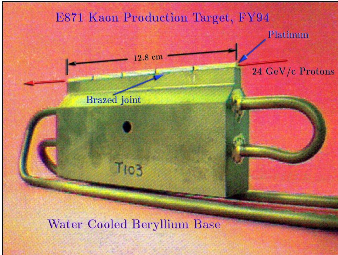
FIG. 19: E871 Production Target
