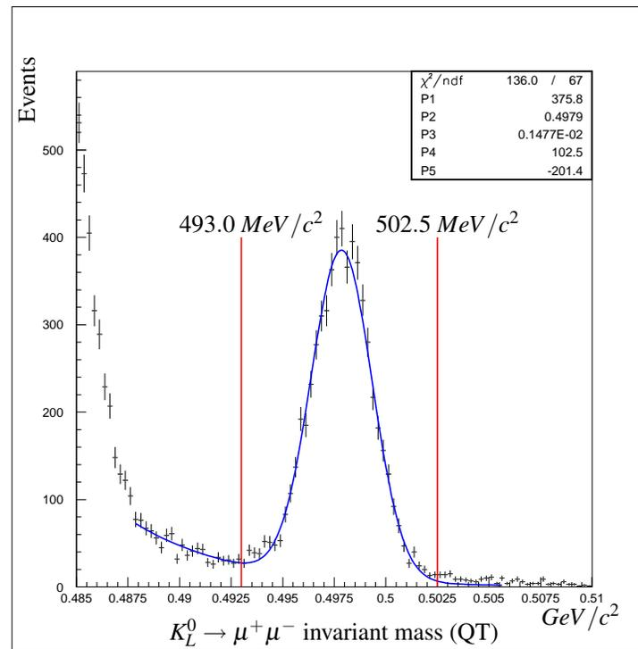
FIG. 49:  $K_L^0 \rightarrow \mu^+ \mu^-$  invariant peak showing 6133 events in the signal region consisting of  $5714 \pm 76$  signal events on an exponential background of  $419 \pm 20$  events.
