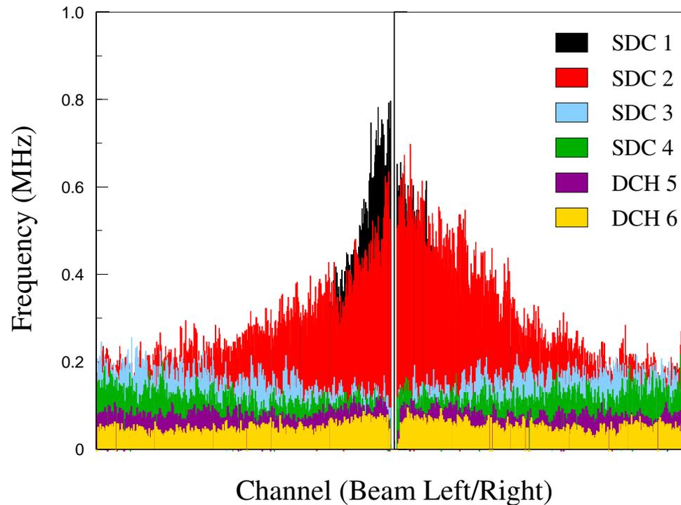
FIG. 22: Signal rate comparison between straw drift chambers and hexagonal drift chambers before and after the neutral beam stop
