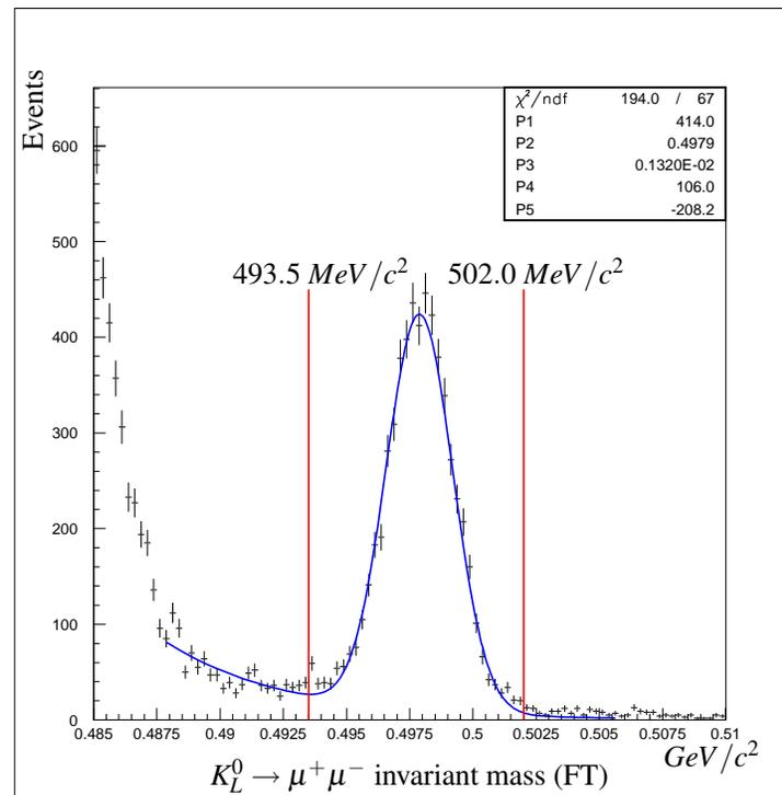
FIG. 48:  $K_L^0 \rightarrow \mu^+ \mu^-$  invariant peak showing 6069 events in the signal region consisting of  $5657 \pm 75$  signal events on an exponential background of  $412 \pm 20$  events.
