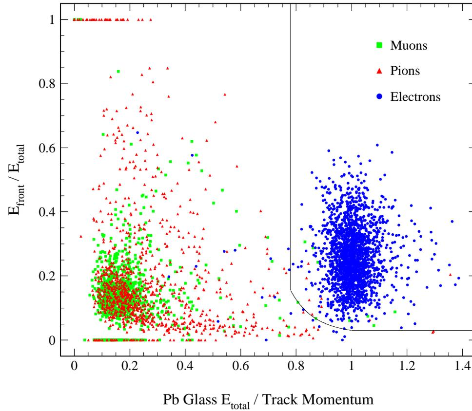
FIG. 27: Lead glass array electron/pion separation contour
