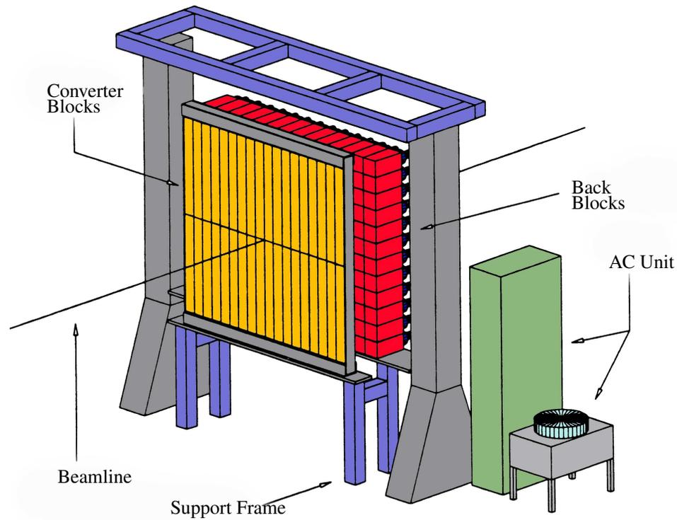
FIG. 26: E871 lead glass array with external cooling system
