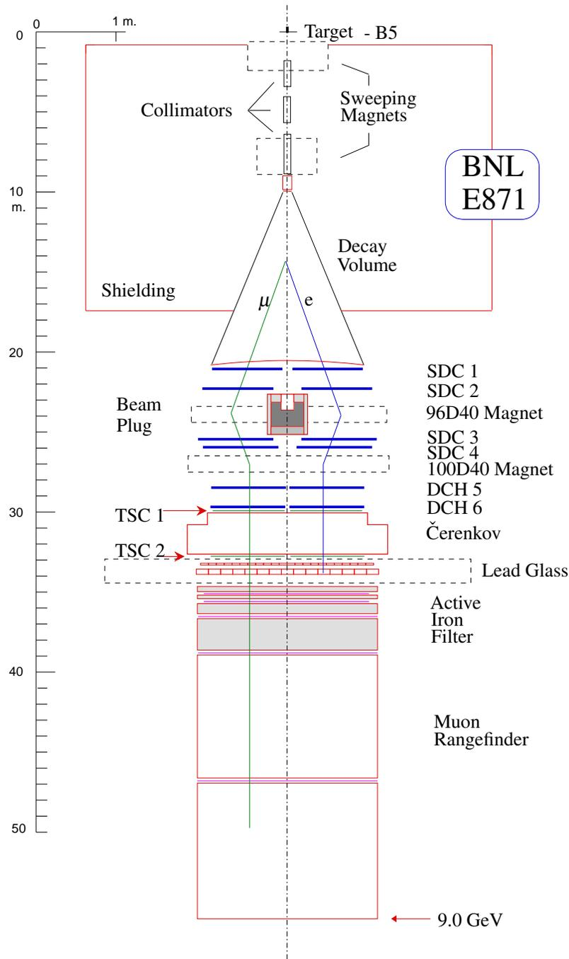
FIG. 18: E871 Spectrometer and particle identification
