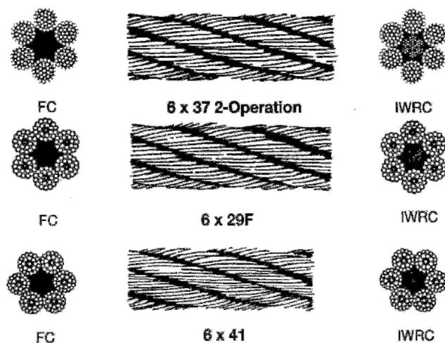
Figure 11-5. 6 x 37 classification of wire rope.
