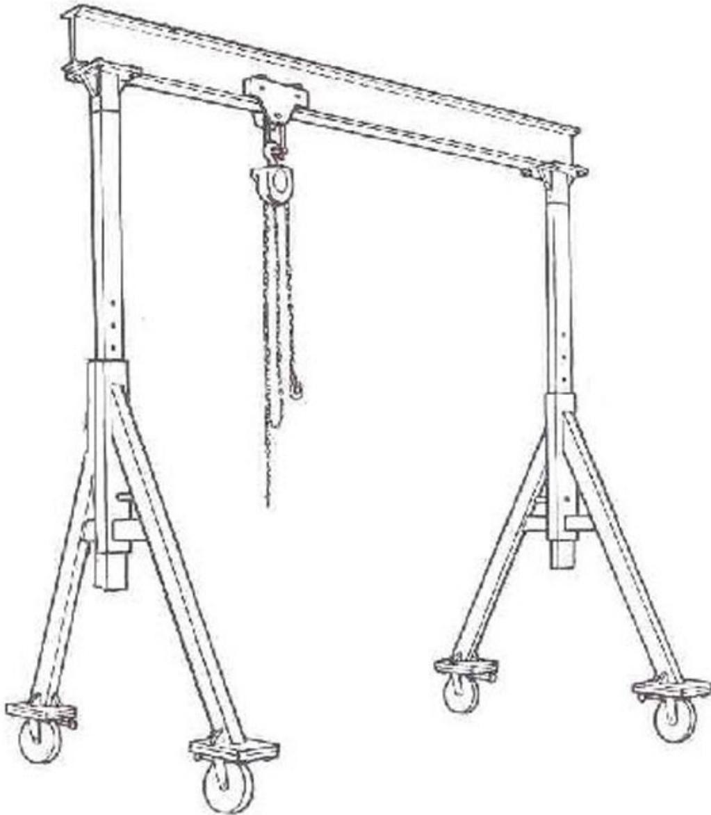
Figure 16-3 Portable A Frame
