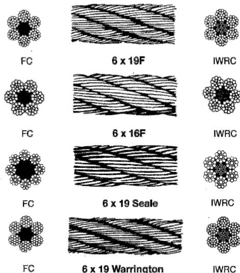
Figure 11-4. 6 x 19 classification of wire rope.
