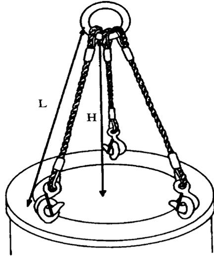
Figure 11-8. Determination of capacity – 3-leg bridle sling.
