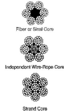
Figure 11-3. Wire-rope cores.
