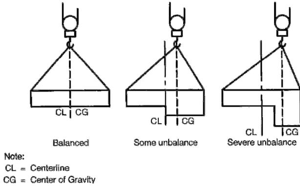
Figure 11-6. Balancing Loads
