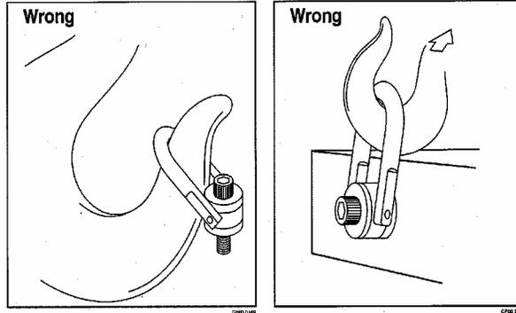
Attach lifting device ensuring free fit to swivel hoist ring bail and ensuring no interference between load (work piece) and bail.
