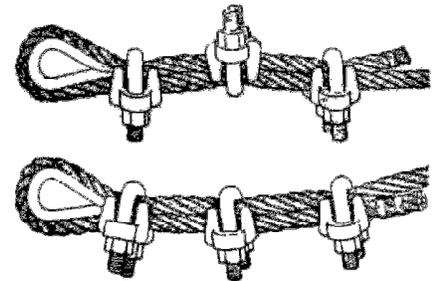
The “U” of the clips shall not bear against the live end of the wire rope because of the possibility of the rope being kinked or crushed.
