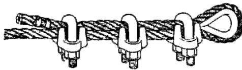
Note that the base of the clip bears against the live end of the wire rope, while the “U” of the bolt presses against the dead end.
