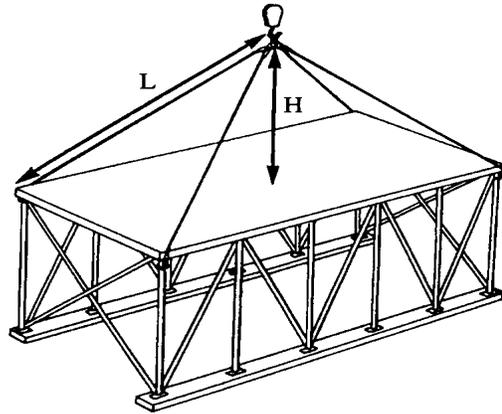
Figure 11-9. Determination of capacity – 4-leg bridle sling.
