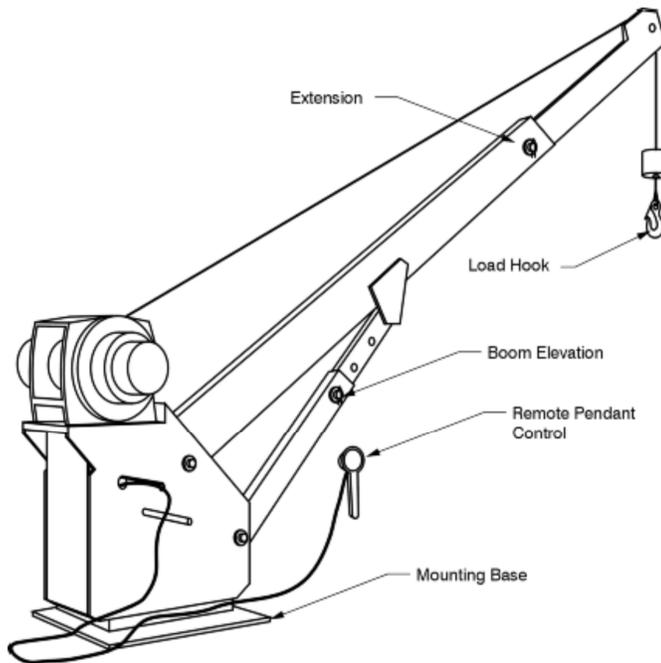
**Figure 16-2. Truck Mounted Crane – Capacity 1 Ton or Less.**
