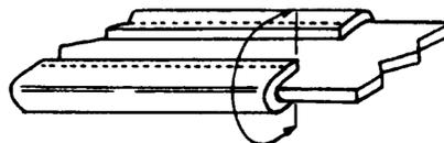
**EDGE GUARD.** A strip of webbing or leather is sewn around each edge of the sling. This is necessary for certain applications where the sling edges are subject to damage.
