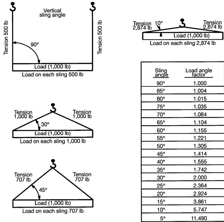
Figure 11-7. Relationship of load angle and lifting efficiency.
