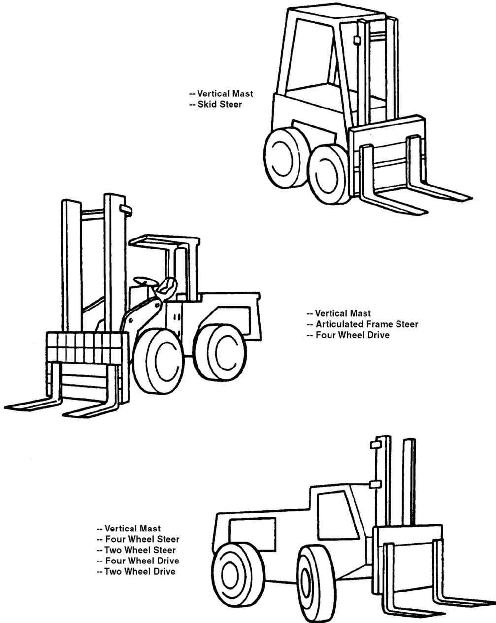
Figure 10-3. Types of Trucks (sheet 3 of 6)
