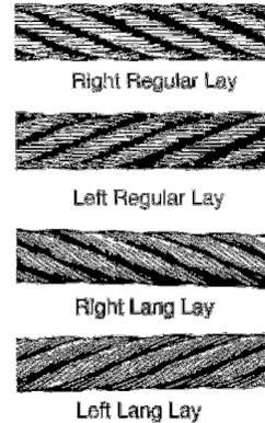
Figure 11-2. Wire-Rope lays.
