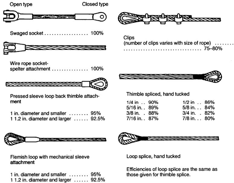
Figure 11-11. Wire-rope fastenings.
