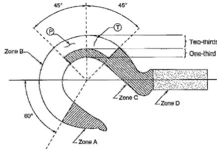
Two directions of discontinuities are labeled on the drawing above as “P” and “T.” discontinuity P parallels the contour of the hook and is considered non-serious in nature and does not require removal from service. Discontinuity T is transverse to contour of the hook and is more serious in nature. Discontinuity T, when occurring in Zones B, C, or D, may reduce longevity of the hook. If the inspection identifies discontinuities, NDT should be considered.
