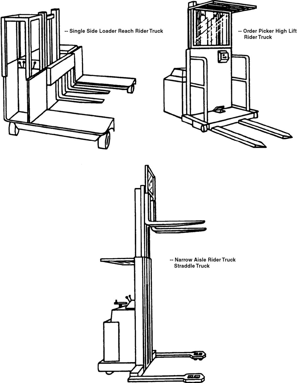
Figure 10-3. Types of Trucks (sheet 6 of 6)
